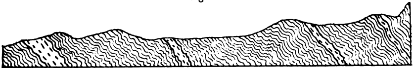
Cross-section through the Evans Gold Property, Cherokee County, Georgia, Showing the Auriferous Quartz Veins in the Crystalline Schists, as Indicated by the Dotted Lines.
